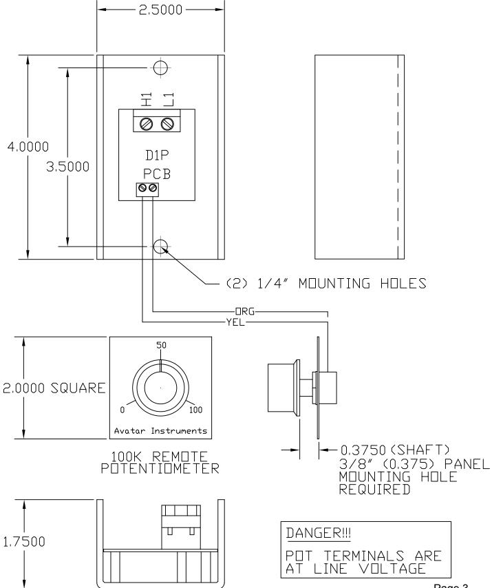
PHYSICAL DIMENSIONS D1P - 30 AMP with remote setpoint potentiometer
